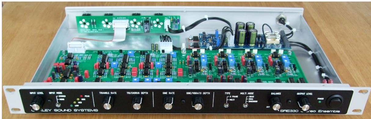
The first prototype unit built into a Bryant Broadcast 1U 250mm deep 19" rack enclosure with the Schaeffer front panel attached. This one used an earlier issue 1 RPSU power module. Issue 2 RPSU boards are green and use a five way 0.156" connector to take power onto the SRE330 main board.
