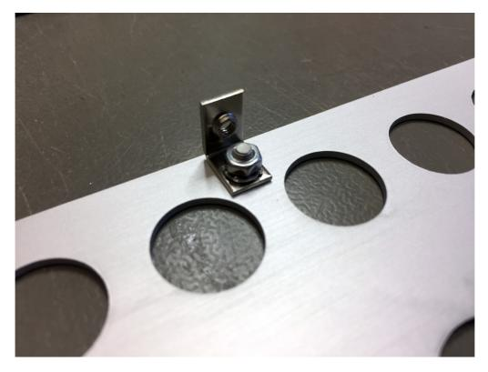
At the forward edge you'll find a use for the M2,5 threaded block with the 3,2mm drilling. Simply attach the block with a M3 female screw and align it properly. Do not break the M3 bolt while tightening the female screw! About 1-1,5mm of the M3 bolt should still stick out.
