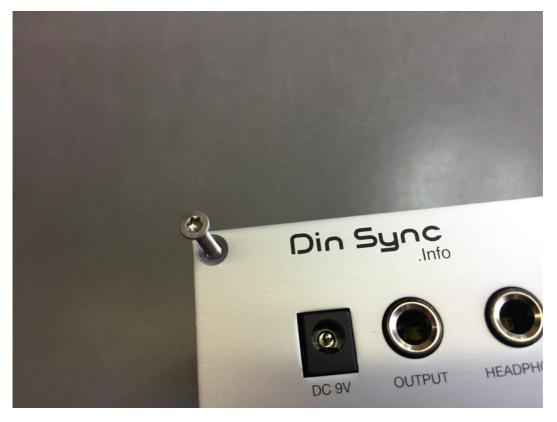
Be cautious while screwing! Be sure to hold the screws in place so they don't accidentally scratch the back panel while being screwed in.
