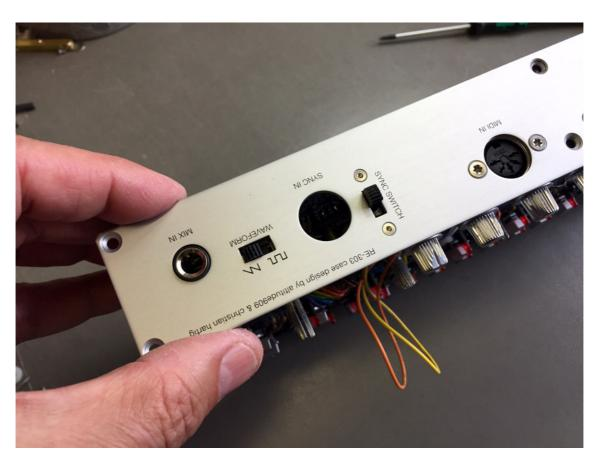
The MIDI jacks should sit perfectly between the axes of the potentiometers.
