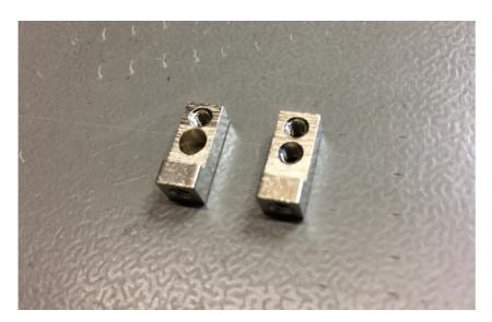
The two M2,5 threaded blocks have a little differnce between the two of them: one has a 3,5mm hole instead of the usual thread. That block is to be attached to the front plate!
