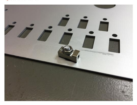
The part oft he M3 bolt, which is sticking out, needs to be filed down: File it down until the bolt sits flush with the female screw. You'll need this additional space for the switchboard!
