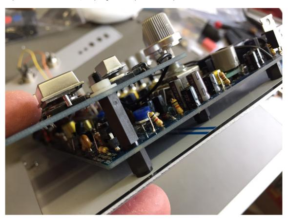
There's still one plastic M3 nut left, which is used to attach the mainboard right next to Q2.
