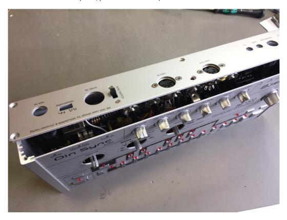
Attach the back panel with the 2,9mm x 19mm tapping screws. It is **NOT** required to drill holes into the side panels! The screws should be screwed directly into the panels!
