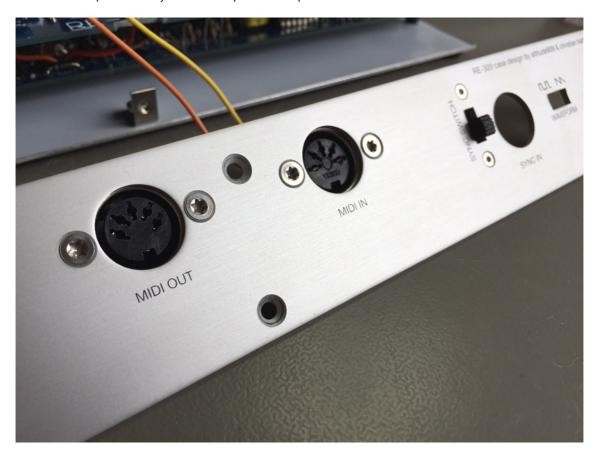
Use the M3x 5mm countersunk screws and M3 nuts to attach the jacks, lock-washers are **NOT** needed!
