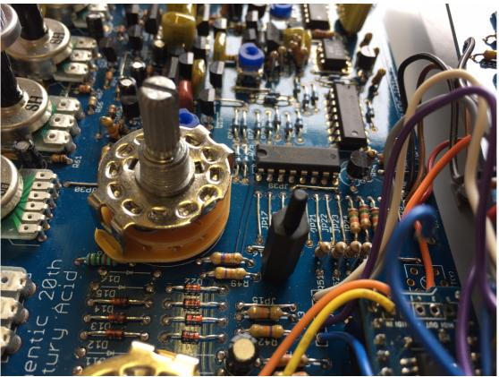
Now you can place the switchboard and attach it with the three plastic washers and three M3 plastic nuts.
