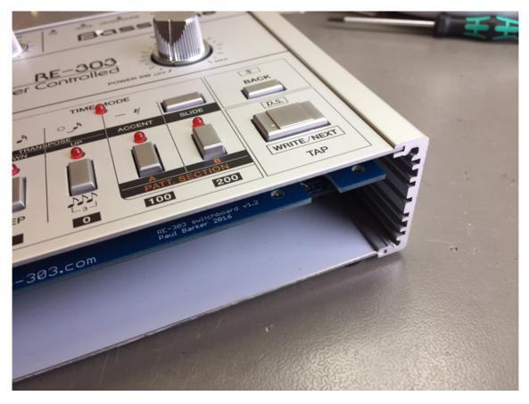
Now the 23mm stand with M2,5 thread is to be screwed to the BACKWARD connector, to support the switchboard.
