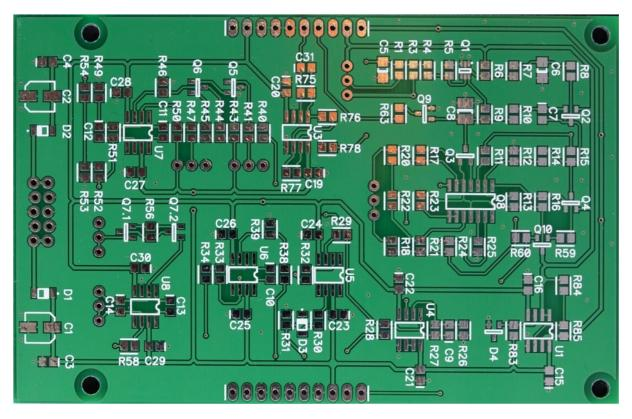
The PCBs are mounted on top of each other, back to back ('sandwich-style'). The 'Back PCB' contains the main circuit, while the 'Front PCB' house the controlling elements, buffers, and the sync-trigger circuit.
