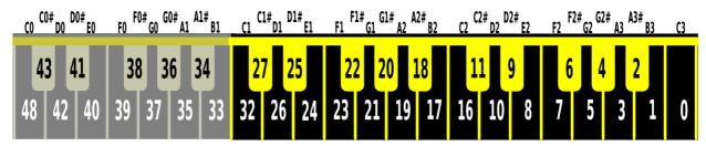
The Wasp/Jasper keyboard allows playing of the top two octaves, but by using the Link port another octave is possible, shown in grey above. There is a hardware 'bug' in the Wasp/Jasper decoding circuitry – the lowest C (C0 above) is not decoded, so it won't play. The Gnat decoding circuitry can play the lowest C.
