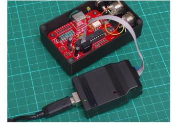
your own code. If you are using an unused blank ATMega328, use the Arduino IDE to flash the Arduino bootloader first. Select Arduino/Genuino Uno as the board type in the IDE.
