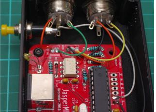
**LED:** The LED can be soldered directly to the PCB if you're making an external box, or it can have wires soldered to its pins so it can be positioned away from the PCB. A standard 2.54mm (0.1") pitch MTA100/MolexKK or JST XH header can be soldered into the LED position on the PCB.
