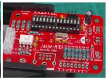
Take care to get the polarity of the diodes, LED and electrolytic capacitors correct. For the LED and electrolytic capacitors the longer (+ve) leg goes into the square shaped pad. Also the negative side of the electrolytic capacitors are shaded on the PCB silk-screen. Before installing the ICs, connect power to the PCB and check that you are getting 5V at the correct places.
